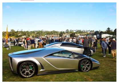
The Kode 0 has a basic structure based on a carbon fiber monocoque with a mid-mounted high-power V12 NA engine. The combination of the 1,550 kg lightweight body, with its extensive use of carbon fiber components, and the high performance engine that delivers 700 hp, provides world-class dynamic performance.
